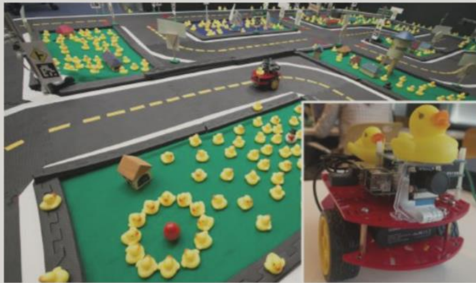
Fig. 1. In Duckietown, inhabitants (duckies) are transported via an autonomous mobility service (Duckiebots). Duckietown is designed to be inexpensive and modular, yet still enable many of the research and educational opportunities of a full-scale self-driving car platform.
